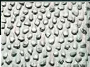
The surface of a STROH ROLLER DRESSER covered by infiltrated and hand set diamond grain (IG type).
